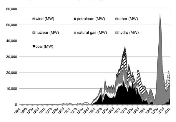
Figure 10: U.S. Power Plant Capacity, by Type and Year It Entered Service
