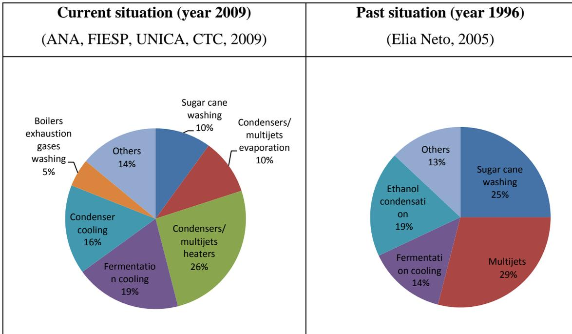
**Figure 2: Water consumption in the sugarcane mills (shares of 22m<sup>3</sup>/ton of cane)**
